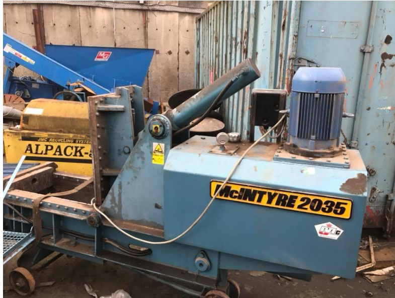
Figure 4: Model of a small compacter machine used to compact wire
